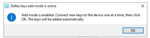
Attach the key to the reader as during authorization - the device will remember the key number - and click "OK". The key number appears in the free field. If several keys are added at the same time, it is allowed to attach them to the reader in turn, while the add window is open, and only then click "OK" - the numbers of all keys will be added to the free fields in the order in which they were applied to the reader.
